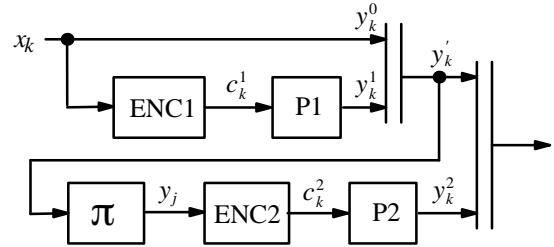
Figure 3: Serial concatenated punctured convolutional (super code) encoder.
