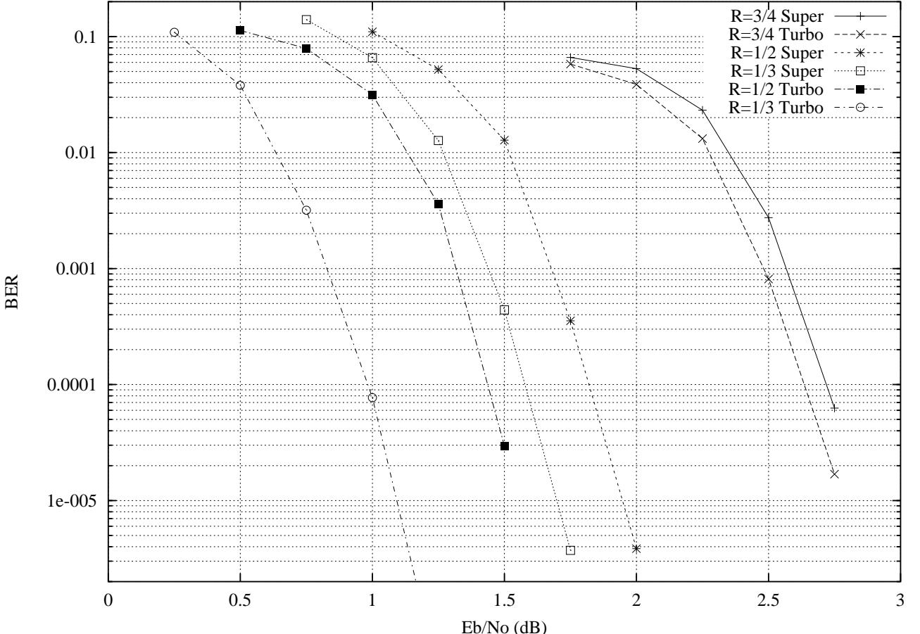
Figure 6: BER for turbo and super codes with 12 iterations.
