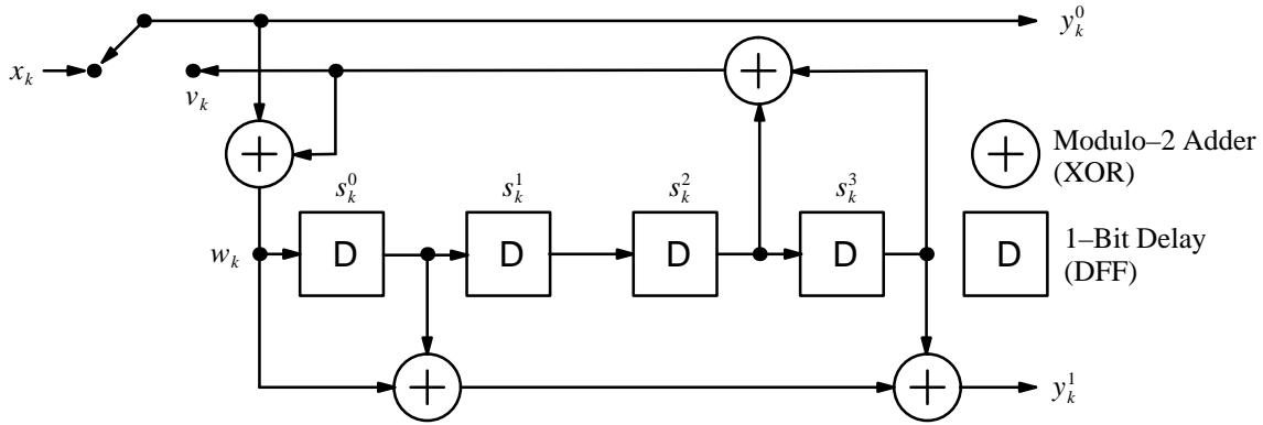
Figure 1: Rate 1/2 16 state systematic recursive convolutional encoder.
