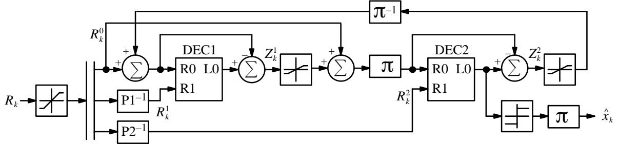
Figure 4: Punctured turbo code decoder.
