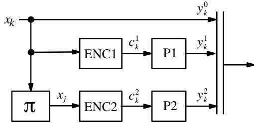
Figure 2: Parallel concatenated punctured convolutional (turbo code) encoder.
