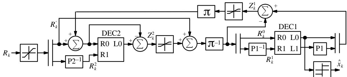
Figure 5: Punctured super code decoder.
