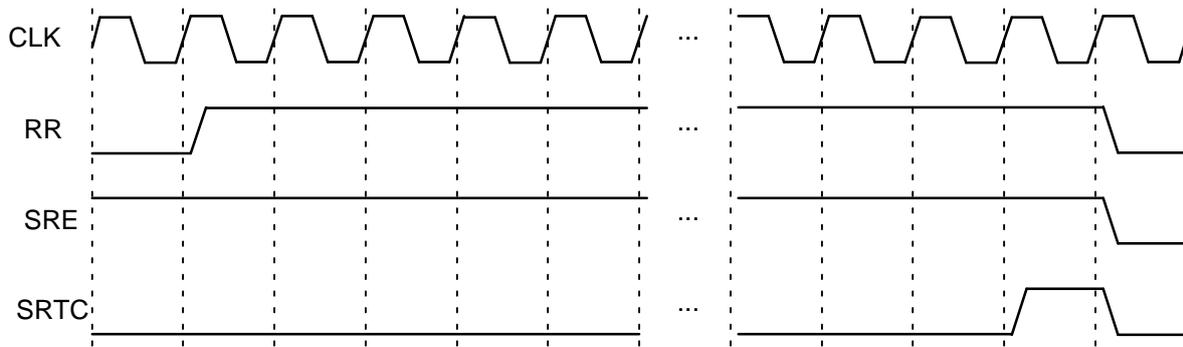
Figure 5: Turbo decoder input timing for last half iteration.
