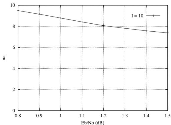
Figure 10: Average number of iterations with block size 1784 and auto-stopping (ZTH = 23).
