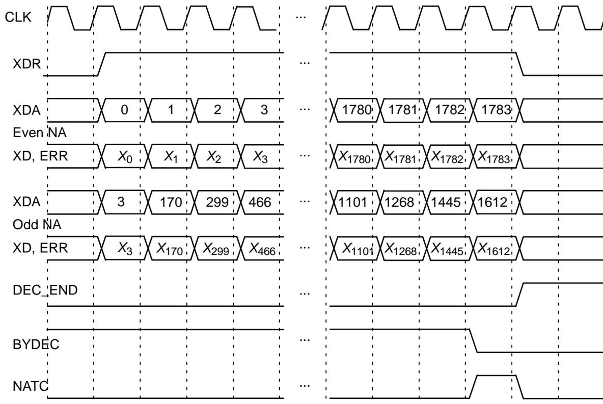
Figure 6: Turbo Decoder Output Timing ( $K = 1784$ ).
