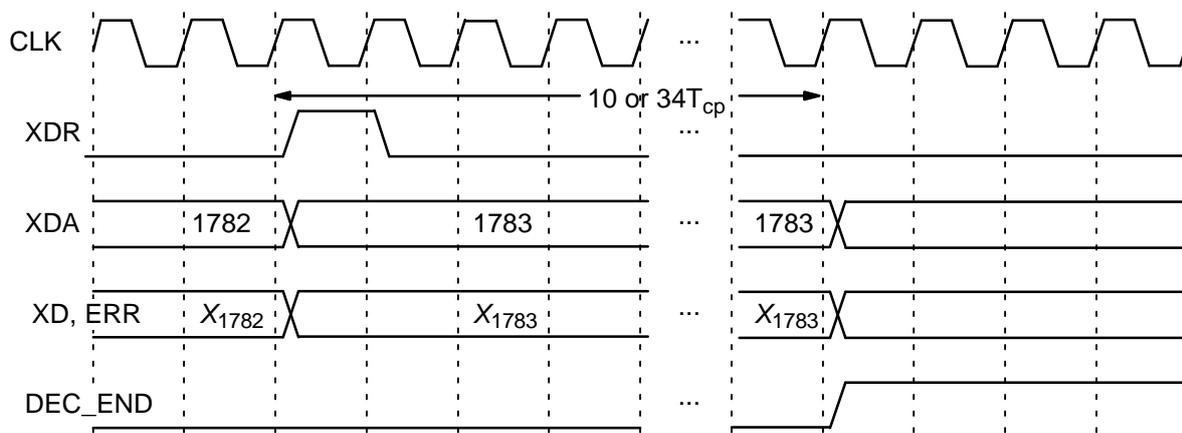
Figure 12: Viterbi Decoder Output Timing (K = 1784).
