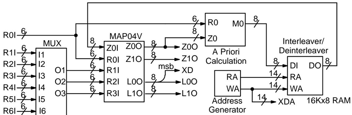
Figure 3: Simplified block diagram of PCD04C 16 state turbo decoder.
