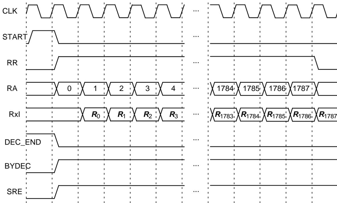
Figure 4: Turbo decoder input timing for first half iteration ( $K = 1784$ ).
