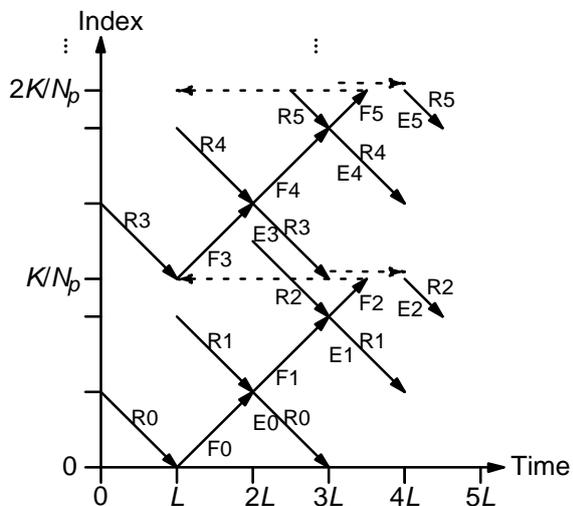
Figure 9: Timing diagram for  $2L < K/N_p \leq 3L$ .
