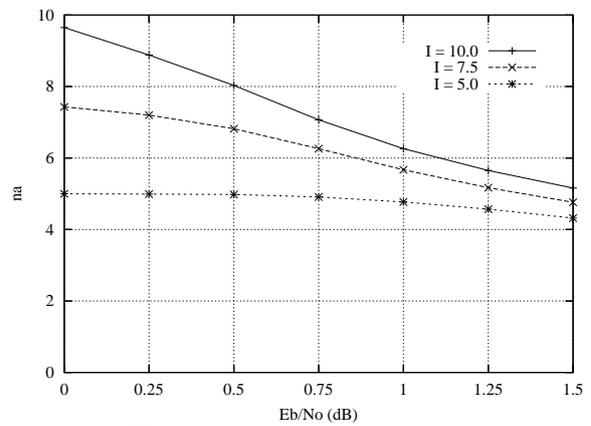
Figure 15: Average number of iterations with  $K = 512$ ,  $N_p = 8$ , log-MAP and auto-stopping.
