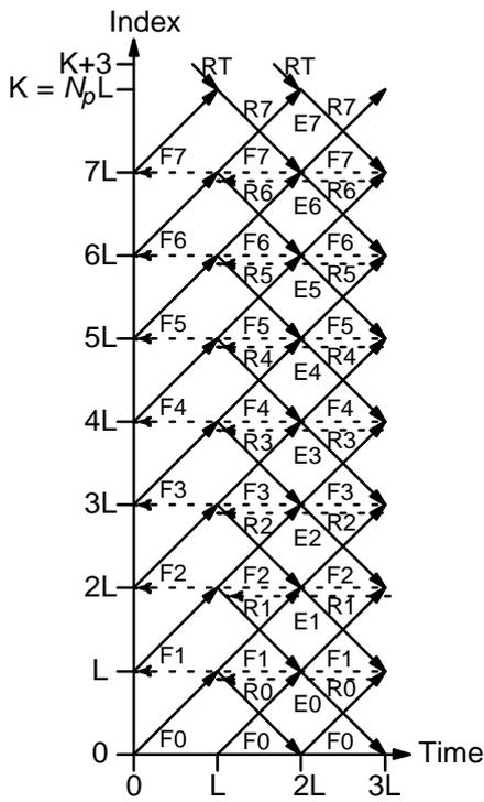
Figure 7: Timing diagram for  $L = K/N_p$ .
