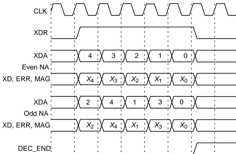
Figure 12: Turbo Decoder Output Timing ( $K = 40, N_p = 8, L = 5$ ).
